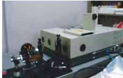
A compact FTIR measures atmospheric \text{CO}_2 concentration.
